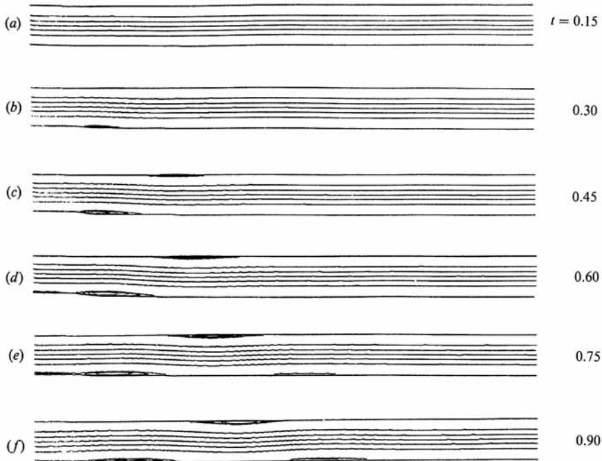
FIGURE 8. Instantaneous streamline plots for a small-amplitude inviscid flow with downstream flow rate fixed ( St = 0.037 , \epsilon = 0.1 ): (a) \psi_{\max} = 1.000 , \psi_{\min} = 0 ; (b) 1.000, -0.003 ; (c) 1.001, -0.009 ; (d) 1.004, -0.014 ; (e) 1.006, -0.015 ; (f) 1.006, -0.009 .
